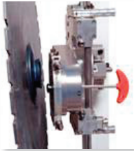
Quick disconnect coupling for blade
