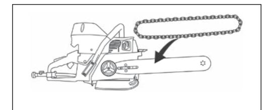
Mount the diamond chain on the guidebar starting at the drive sprocket and continue over the guidebar nose.
