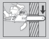
3. Insert WallWalker® rotate rear handle up
