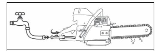
Attach to water supply capable of delivering 1.5 bar (20 psi) pressure to the saw at a minimum flow rate of 4 lpm (1 gpm). The single most important factor an operator can control to increase chain life is to use adequate water pressure.
