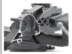
20.30 Slide the clutch side shaft through the bearing.
