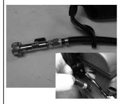
15.2 Release clip from water inlet pipe. Pull hose upward.
