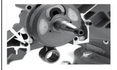
Lubricate the crankcase halves with ICS<sup>®</sup> 2-stroke oil and install the crankcase gasket.
