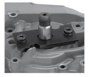
20.15 Attach universal puller and press out the crank shaft.
