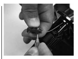
18.9 Remove throttle cable through the front of the handle.
