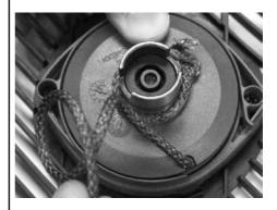
9.6 Remove the center screw and components.
