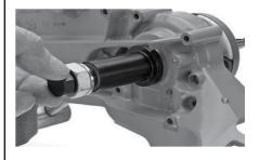
Slide the shaft sleeve over the shaft, against the crankcase. Thread the M12 mandrel with the nut and washer until it bottoms (Note - **REVERSE THREAD** on the clutch side).
