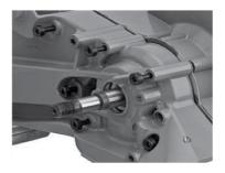
Tighten the screws to 106 - 124 in-lbs./ 12 - 14 Nm using an "x" pattern.
