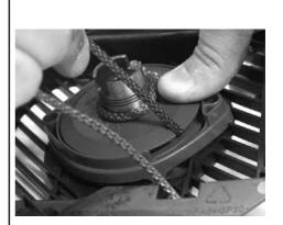
9.5 Pulley removal from spring.
