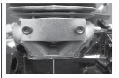
25.5 Install the intake seal flange.
