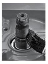
20.7 Install the new seal. Use caution as seal slides over the threads.
