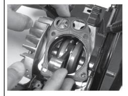
16.11 Lubricate needle roller with ICS<sup>®</sup> 2-stroke oil. Insert into the connecting rod.
