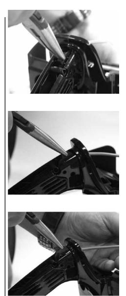
18.7 Remove cable lever (P/N 543814) using needle nose pliers pulling up.
