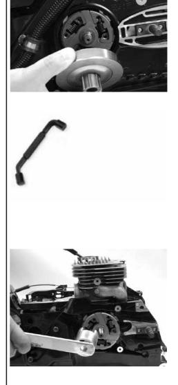
8.8 Remove clutch with clutch tool (P/N 546659).
