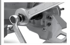
20.33 Install the (2) crankcase guide pins.
