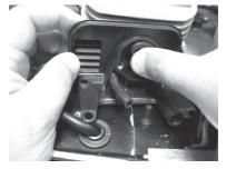
Remove pulse tube and protective spring from cylinder base.
