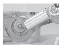
Remove the flywheel side crankcase — tap crankshaft with plastic mallet.
