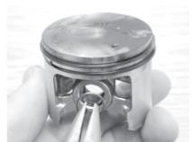
Make sure wrist pin retaining clip is in the proper orientation.
