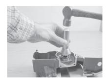
Install crankshaft into clutch side of case.
