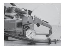
The fuel tank breather stabilizes the pressure in the fuel tank preventing both excessive pressure, which could flood the engine, and negative pressure, which could starve the engine of fuel.
