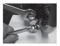
Unscrew water tank cap from the power cutter (7/8 wrench).
