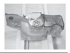
Align crankcase gasket on flywheel side crankcase pins.
