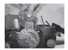
Install 4 cylinder screws and washers.
