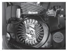
16. This section covers the removal, inspection, and installation of the flywheel. Removal of the starter and spark plug is required. Refer to sections 6 and 8 if necessary.
