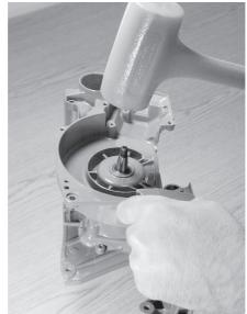
19.5 Remove the flywheel side crankcase seal with 1/2" (13 mm) socket.
