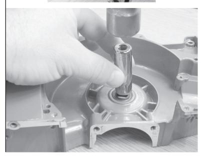
19.6 Disassembly of crankcase.Heat the clutch side crankcase with heat gun to 150° F (65.5° C).
