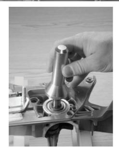
19.17 Coat crankcase gasket with ICS® 2-stroke engine oil.
