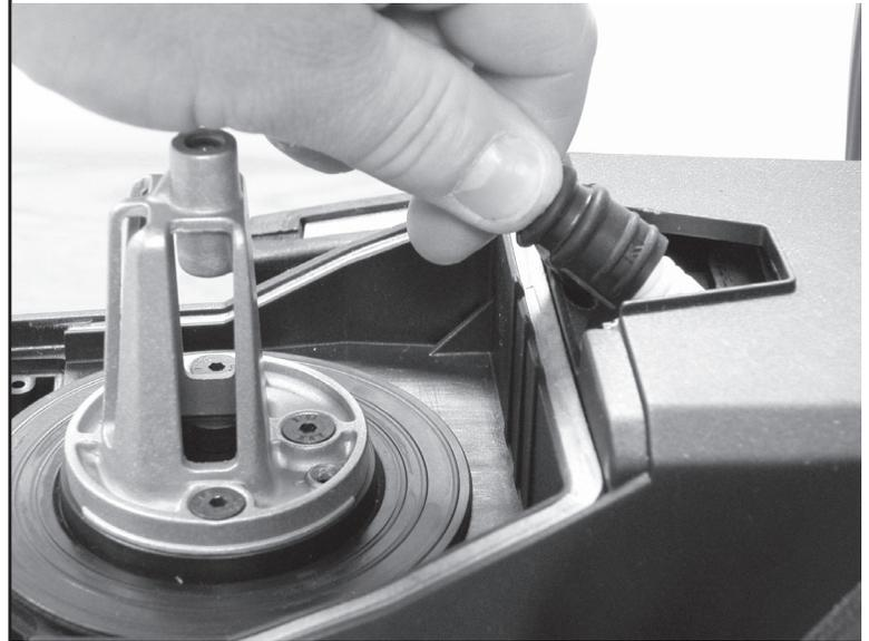
7 This section covers clutch removal, rim sprocket removal, inspection, and assembly. Refer to sections 5 and 6 if necessary.
