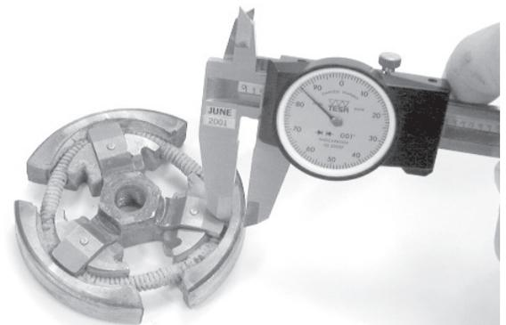
7.7 Inspect spring for cracks.
