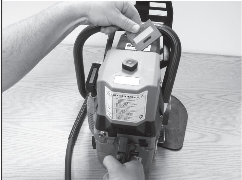
23.11 When the carburetor is adjusted correctly set the limiter caps with a  $\frac{1}{4}$ " straight blade screwdriver.
